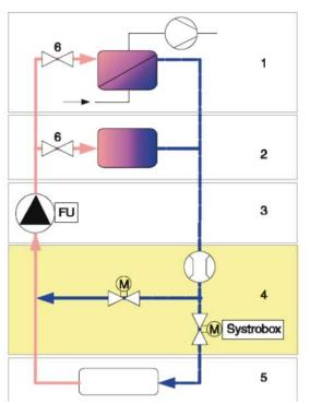
Schematic of heating/cooling circuits
