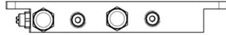
Base for actuators with VDI/VDE 3845 interface, not applicable to ACTAIR and DYNACTAIR
